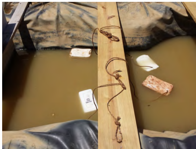
Figure 2-3: Photograph of four 703d type Floc Logs suspended in the turbidity test channel. One control (no Floc Log) and two tests (with Floc Logs) were completed: the first test used one 703d Floc Log and second test used four 703d Floc Logs (Figure 2-3); the Floc Logs were placed between the sampling locations at the front and middle of the channel.
