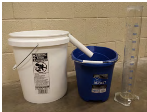
Figure 2-6: Photograph of the equipment used to measure the volume of the Floc Logs, which includes an overflow bucket (on the left), a catch bucket (center frame), and a graduated cylinder (on the right).
