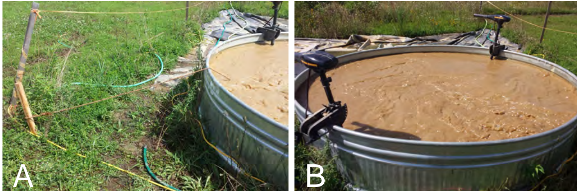
Figure 2-4: Photographs of the basin-scale jar tests. (A) Photo of the Floc Log roped around a stake and suspended in the turbid water tank, (B) Photo of the stock tank filled with turbid water with the two trolling motors attached.
