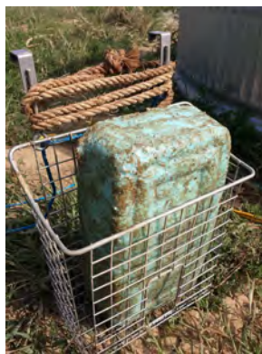
Figure 2-5: A single 703d#3 Floc Log placed inside of a cage container used for the eight consecutive basin-scale jar tests.
