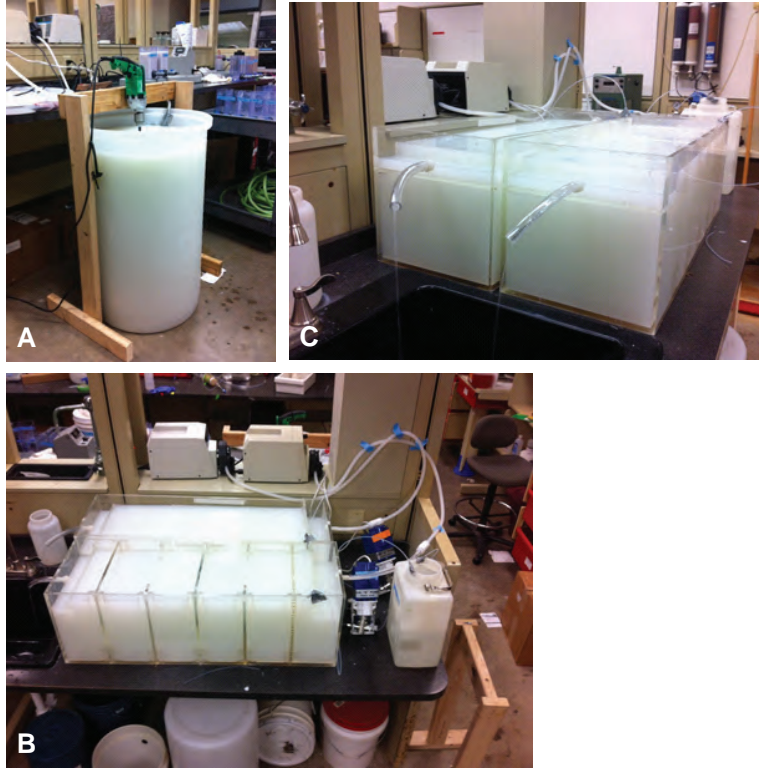
Figure 2-1: Photographs of the Phase II lab-scale hydraulic flocculation setup. (A) a 200 L bucket filled with tap water amended with 2 \text{ g L}^{-1} kaolinite mixed at constant speed with a paddle controlled by a drill, (B) two 65 L flow through reactors (baffled reactor in the foreground), two peristaltic pumps (in the background) to supply the turbid water to the reactors, and a 9 L carboy containing PAM stock solution supplied to the reactors with a piston pump (to the right of the reactors), and (C) effluent of the two 65 L reactors.
